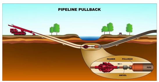
HDD is used for the installation of pipes and utility lines and is characterised by its use of a surface-mounted drill rig that launches and places a drill string at a shallow angle to the surface and has tracking and steering capabilities.
