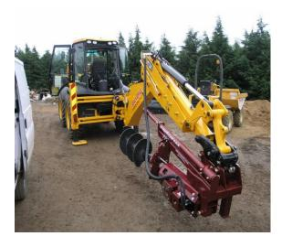
With the advancement of technical equipment, there is increasing use of excavator mounted augers. These can be used application where it is required to bore under shorter crossings such as under other utilities. This would involve open cut trenching up to the required bore on each side and then lowering in the auger into the open trench to undertake the bore.
