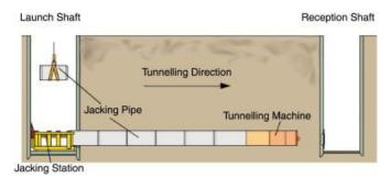
Microtunnelling, sometimes called closed face boring, is a form of trenchless construction that employs a remotely operated microtunnelling boring machine.
