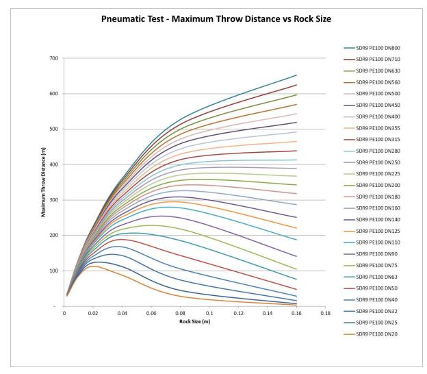
SDR 9 PE100. at Test Pressure of 2.5 MPa (full bore rupture).
